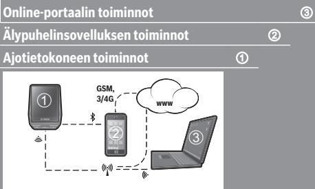
The diagram illustrates the communication network. It shows three main components: a bicycle computer (1), a smartphone (2), and a laptop (3). The bicycle computer is connected to the smartphone via Bluetooth. The smartphone is connected to the laptop via a GSM/3G connection. The laptop is also connected to the internet (WWW).
