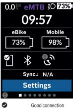
As well as the status bar, the status page also shows you the current time and the state of charge of all your eBike's batteries, as well as the state of charge of your smartphone battery if the smartphone is connected via *Bluetooth*<sup>®</sup>.
