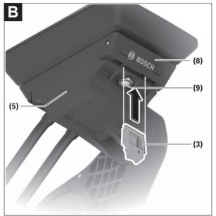
**Note:** Depending on the design/mounting of the display mount, it may not be possible to insert the removal blocker. The display must be mounted. Insert the removal blocker (3) into the adapter tray (5) from below until you hear the removal blocker (3) click into place.
