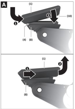
To fit the display (1), attach the display (1) to the front edge of the display mount (8) in the direction of travel, on the snap-in hook (4) • and press the rear side of the display (1) on the display mount (8) •.
