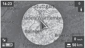
The basic remaining range of the battery can be extended by means of the **"Topo operating range"** premium feature. The **"Topo operating range"** feature then calculates and displays the battery's remaining range, taking into consideration the topographical conditions. The calculation of the topographic range extends to 100 km maximum.
