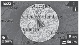
The basic remaining range of the battery can be extended by means of the **"Topo operating range"** premium feature. The **"Topo operating range"** feature then calculates and displays the battery's remaining range, taking into consideration the topographical conditions.
