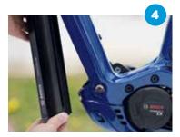
Remove the battery from the frame.
