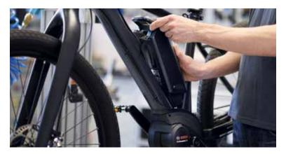
**PowerTubes** – The PowerTubes move approximately 2 cm out of the frame when unlocked, making them easier to handle. In addition, a safety mechanism prevents the batteries from falling out. The batteries are also protected by the frame.
