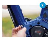
When the battery is unlocked using a key (depending on the manufacturer), it automatically drops into the restraint support.
