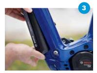
Push the top of the battery to detach it from the restraint support – the battery then drops into your hand.
