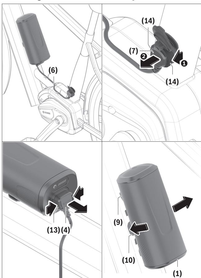
Firstly, disconnect the cable (6) by opening the cable lock as directed by the eBike manufacturer.
