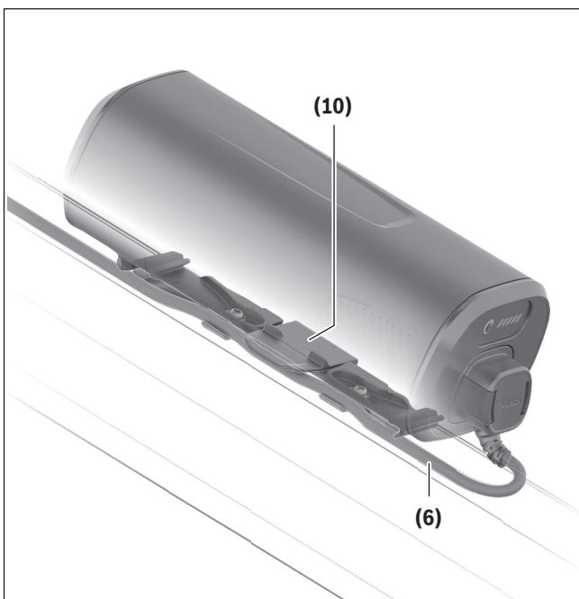
**Note:** When laying the cable (6), make sure that the cable (6) is fed under the release button (10). This prevents the release button (10) from being pressed accidentally and causing the PowerMore battery to be released.
