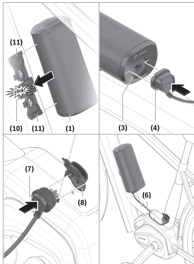
To **insert** the battery (1), place its guide grooves (12) onto the guide rails (11). Ensure that the battery is aligned correctly and that the battery is
