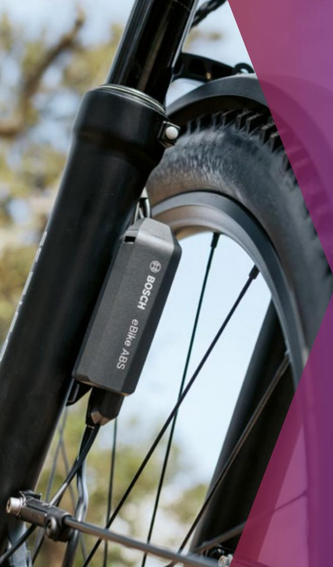
A close-up photograph of a bicycle's front wheel and fork. A black Bosch eBike ABS sensor is mounted on the fork. The sensor has the Bosch logo and the text 'BOSCH eBike ABS' printed on it. The background is a blurred outdoor scene with trees.
